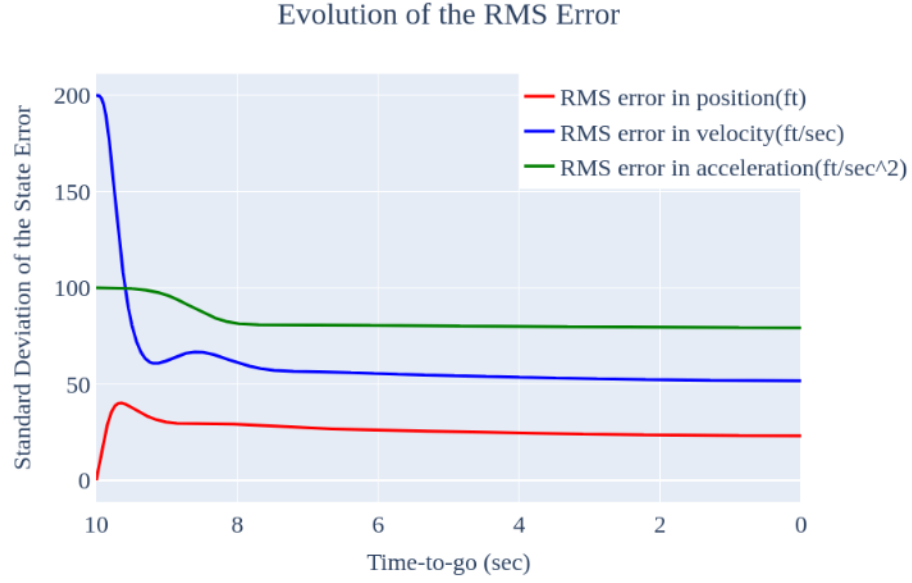
Figure 3: The evolution of the RMS error computed a priori.
